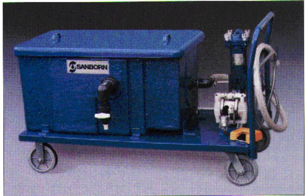
The Sanborn Oil Separator allows coolant to be continuously cycled from the sump or central system to the unit where it is processed and returned as clarified fluid, while the tramp oils are automatically discharged for collection. Two configurations are available with processing capacities of 5 GPM and 10 GPM.
