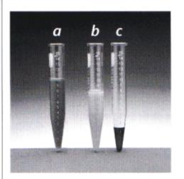
Photo shows (a) dirty coolant before it is processed by the Sanborn Oil Separator and (b) coolant as it is returned to the sump after processing.
