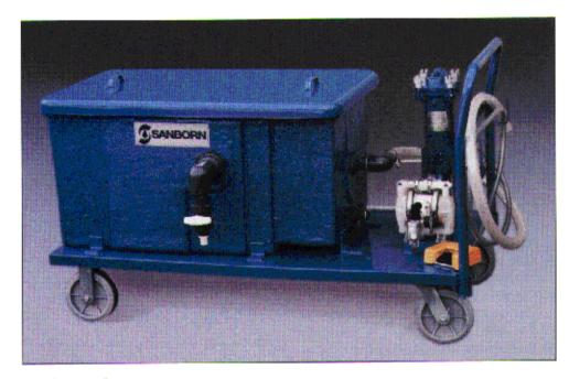
The Sanborn Oil Separator allows coolant to be continuously cycled from the sump or central system to the unit where it is processed and returned as clarified fluid, while the tramp oils are automatically discharged for collection. Two configurations are available with processing capacities of 5 GPM and 10 GPM.
