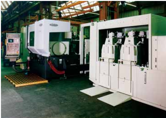
Pictured: Dual T40 Automatic Discharging Centrifuges Processing Rate 80 GPM
