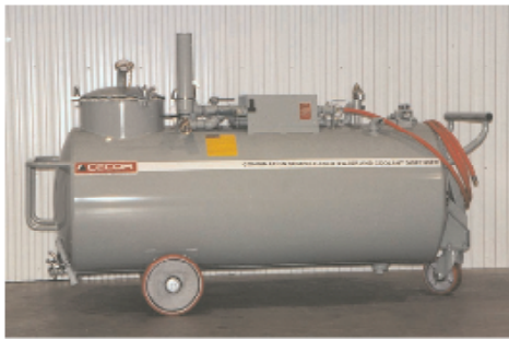
CAS-100/100PT Sumpcleaner/Filter and Coolant Dispenser.
